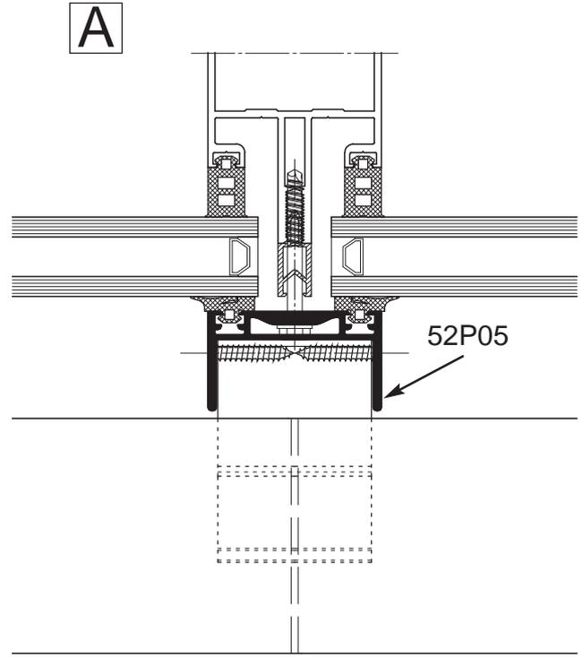
Allow 1mm expansion joint for every 1m length of blade. All expansion joints to be centrally located about a mullion.
