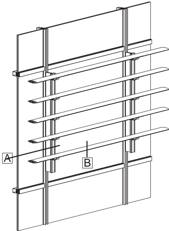
Allow 1mm expansion joint for every 1m length of blade. All expansion joints to be centrally located about a mullion.
