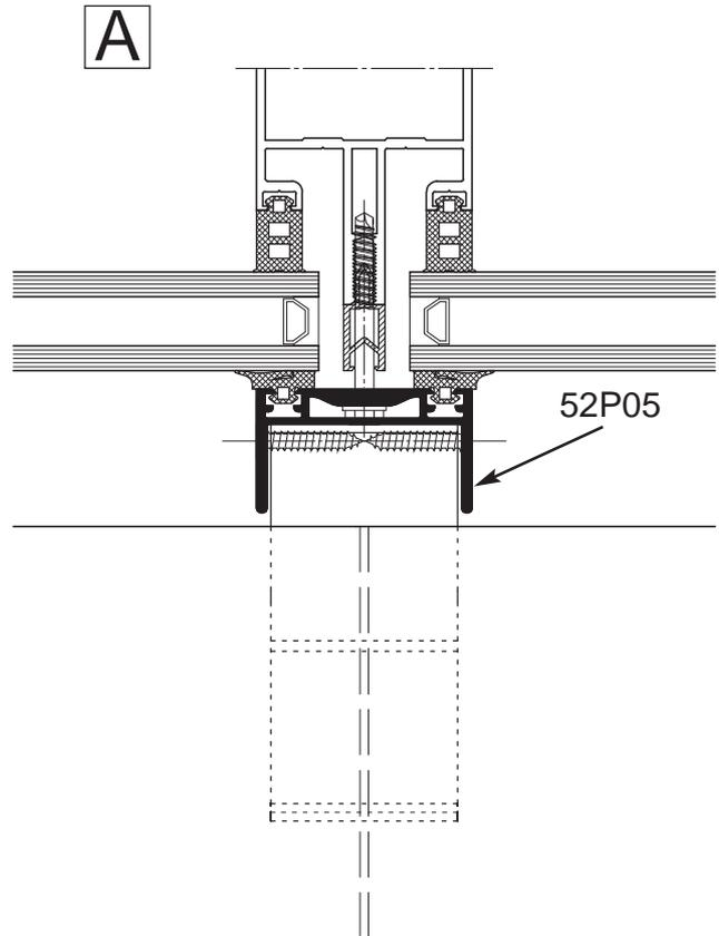
Allow 1mm expansion joint for every 1m length of blade. All expansion joints to be centrally located about a mullion.
