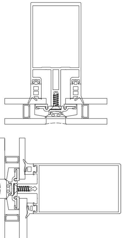
Elegance 52 SG is a structurally glazed curtain wall system using the basic substructure of Elegance 52 and offering a solution for combinations of fixed or opening panels in both straight or faceted applications. The structurally glazed curtain wall offers a minimal sightline without having a visual difference between fixed and opening panels.
